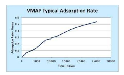
This chart indicates the rate of moisture adsorption of VMAP when exposed to conditions of 50% RH at 22°C sample size 50mm x 30mm x 8mm
