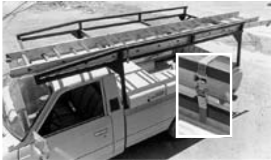
A. Secure ladders and other equipment to trucks.
