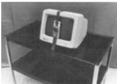
F. Secure delicate equipment to carts for in-plant movement.
