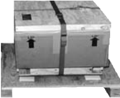
I. Secure cargo to floating platform in wooden shipping crate.
