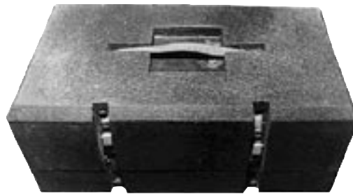
L. Straps can be used to secure contents inside container or can. Replace latches and hinges on outside of container.
