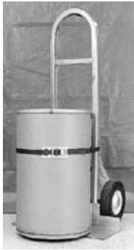
K. Secure equipment or material to handcarts and dollies.
